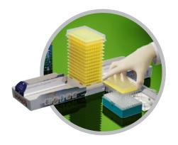
Align Snapload<sup>™</sup> transfer top over refillable rack and place onto rack.
