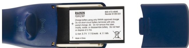
Figure 5: Installing the main battery
