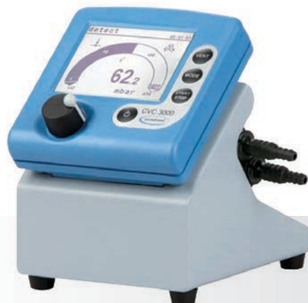
The CVC3000 detect vacuum controller can let you select a setpoint, run a complex program 'ramp' or even automatically find the first boiling point. It works with benchtop diaphragm pumps from all manufacturers.
