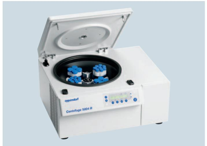
Centrifuge 5804 R with rotor S-4-72 (4 x 250 mL)
