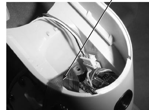
Figure F.3.2g: Unclasp Battery Connector
