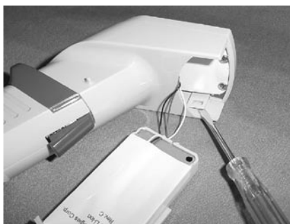
Figure F.3.2c: Unclip Snaps
