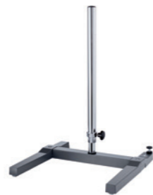
R 2723 Telescopic stand Particularly stable stand with H-shape base which prevents the stand from tipping backwards. Additionally equipped with a pneumatic spring stand rod, which enables heavy instruments/attachments to be raised and lowered smoothly without difficulty. Height: 620 - 1010 mm. Ident. No. 0001412100
