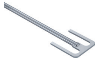
R 1330 Anchor stirrer Tangential flow, high shearing rate at edges, minimum deposits on the vessel wall. Used at low speeds. Polymer reactions, even distribution of high mineral contents in liquids. The ideal stirrer for medium to highly viscous fluids. Ident. No. 0002022300
