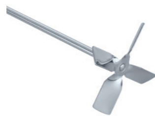
R 1345 Propeller stirrer, 4-bladed Standard stirring element. For drawing the material to be mixed from the top to the bottom. Local shearing forces. Generates axial flow in the vessel. Used at medium to high speeds. Ident. No. 0000741300
