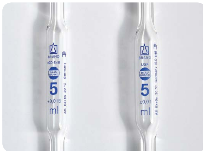
Fig. 3: Examples for inscriptions of 5 ml transfer pipet in accord with ISO (left) or USP/ASTM (right)
