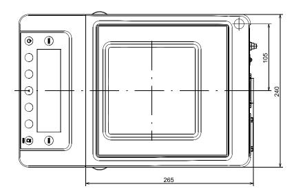
**Precision High Capacity Balances**All dimensions are given in millimeters
