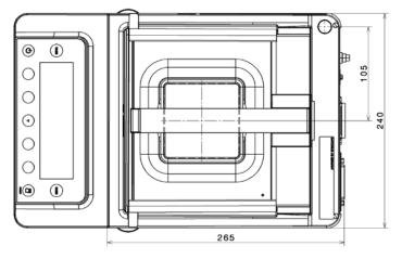
Draft shield DU interior dimensions  $\label{eq:constraint} \mbox{(H)261} \times \mbox{(W)193} \times \mbox{(D)191}$
