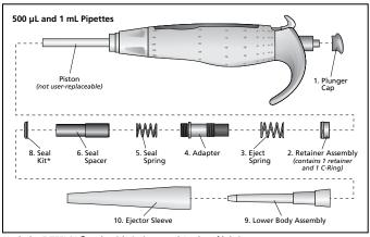
\*Includes 5 TEFLON® seals with O-rings, and 1 tube of lubricant.
