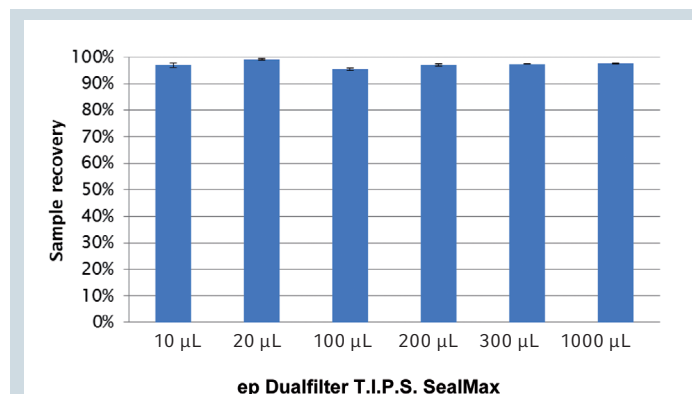
Figure 2: Sample recovery rate of ep Dualfilter T.I.P.S. SealMax following over-pipetting of water. Values presented are average percentage of sample recovery calculated from 10 individual measurements. The error bar represents standard deviation.
