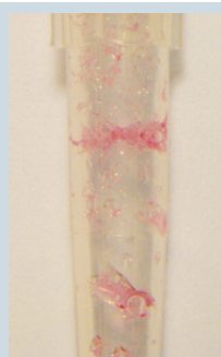
Figure 4: Sample liquid became slightly viscous and had tendency of foam formation after coming into contact with the filter (filter tip from one of the two other manufacturers tested). This observation was made during the investigation, in which distilled water (colorless) was used as test liquid. For visualization, the picture shows test using distilled water with added red dye.
